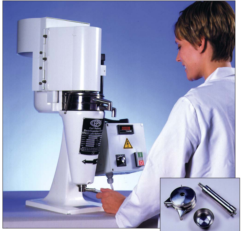
Model LE Benchtop centrifuge for lab scale separation of process volumes from 1.5 to 15 liters. Accessories are easily added or removed without need for tools, for rapid set up and clean up.
