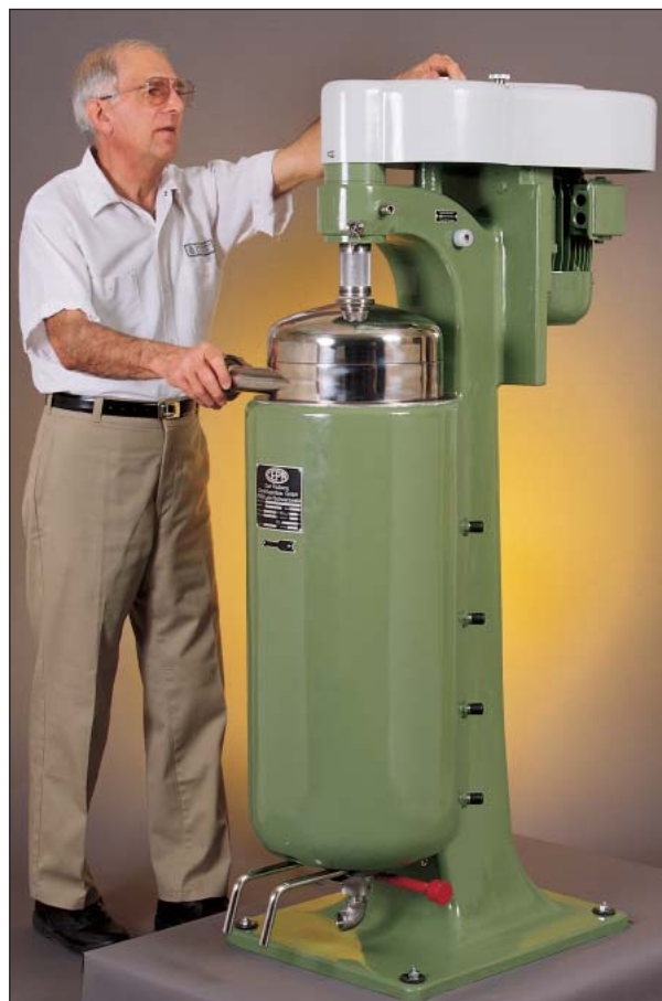
Model Z81, a large production centrifuge, processes volumes from 100 to 2,000 liters depending on solids content.
