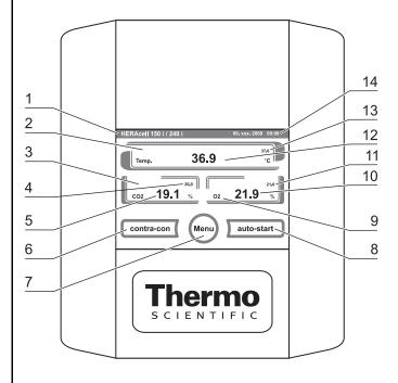
Fig. 33: iCan<sup>™</sup> touchscreen with combined gas connection
