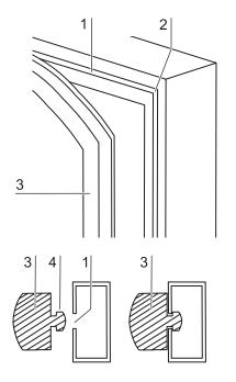
Fig. 77: Magnetic door seal replacement
