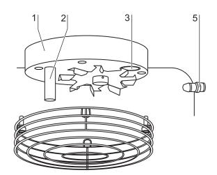
Fig. 11: Temperature,  $CO_2$ , and  $O_2$  sensors
