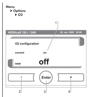
Fig. 58: Switching the O2 control on and off
