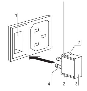
Fig. 76: Device fuse replacement
