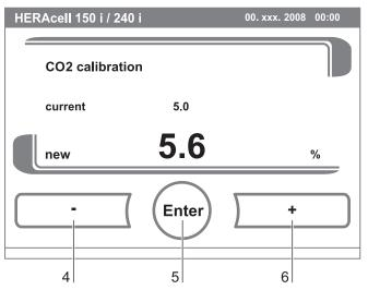
Fig. 74: CO<sub>2</sub> calibration procedure
