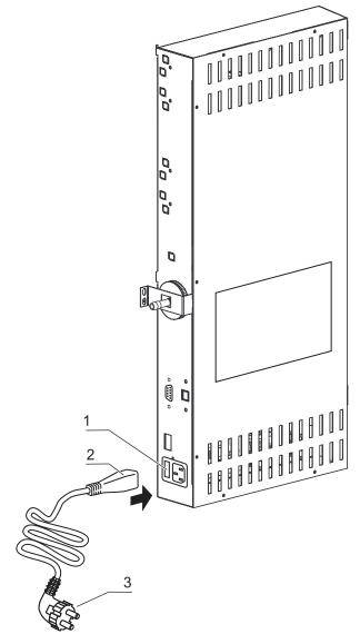
Fig. 28: Power supply connection
