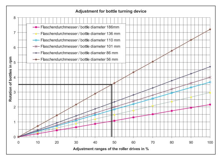
Fig. 22: Bottle turning speed
