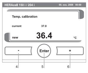
Fig. 71: Temperature calibration procedure
