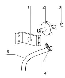
Fig. 75: Gas inlet filter installation
