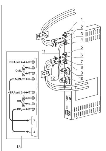
Fig. 27: Combined connection with gas monitoring system (optional)
