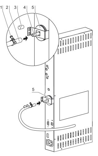
Fig. 24: Installing gas pressure hoses
