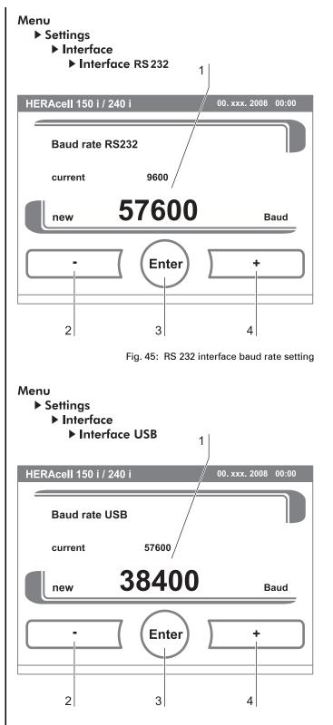
Fig. 46: USB interface baud rate setting
