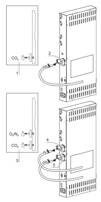
Fig. 25: Gas connection without gas monitoring system
