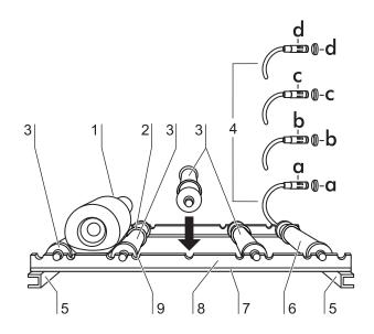
Fig. 21: Installing the bottle turning devices
