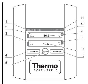
Fig. 32: iCan<sup>M</sup> touchscreen withoutO<sub>2</sub>/N<sub>2</sub>gas supply
