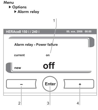
Fig. 52: Alarm relay setting
