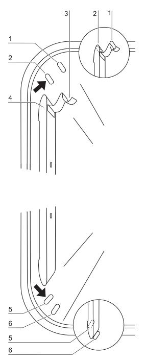
Fig. 18: Support rail installation/removal
