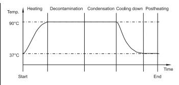
Fig. 66: Decontamination routine phases
