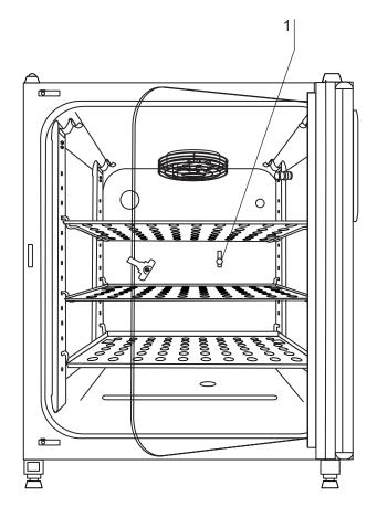
Fig. 72: Preparing  $CO_2$  calibration
