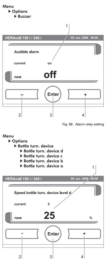
Fig. 57: Bottle turning device speed setting
