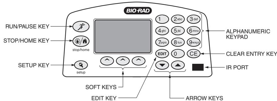
Fig. 4. Front Panel.
