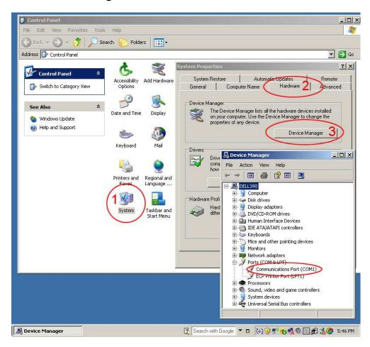
Before interfacing with a PC, make sure a RS232 port exists on your PC. RS232 ports will be in parentheses and named "COM1-100" like the one above named COM1
