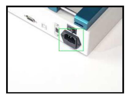
Step 2: Remove the fuse holder from the power plug. There is a small indentation on the bottom edge of the power plug. A small coin or screw driver may be needed to remove the fuse holder from the pump.
