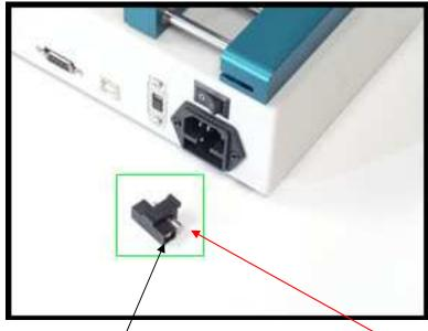
There are 2 fuses in the fuse holder. The exposed fuse in the back is the fuse that is being currently used. In the event of a power surge this fuse will be the broken fuse.
